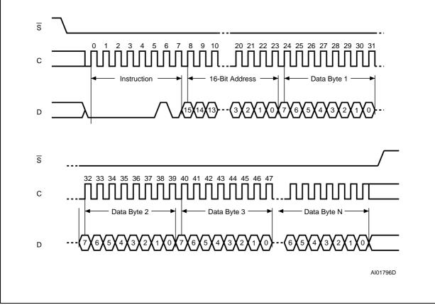
Note: Depending on the memory size, as shown in Table 6, the most significant address bits are Don't Care.
