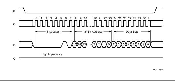
Note: Depending on the memory size, as shown in Table 6, the most significant address bits are Don't Care.
