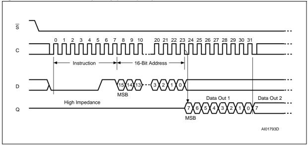
Figure 11. Read from Memory Array (READ) Sequence
